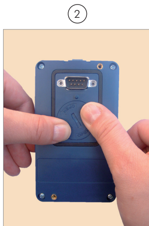
Press the cover and rotate it counterclockwise
