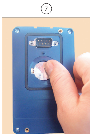
Press the battery for its insertion
