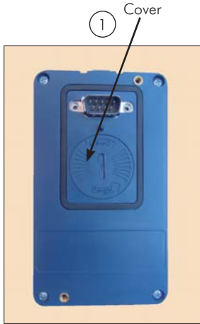
Location of the battery access cover
