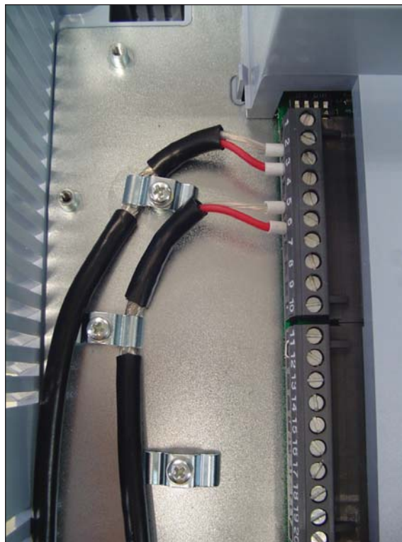
Figure 3.16 - Example of control wiring shield connection
