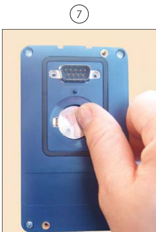
Press the battery for its insertion
