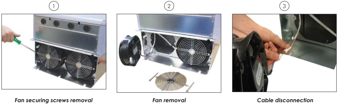
Figure 6.1 - Removal of the heatsink fans
