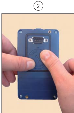
Press the cover and rotate it counterclockwise
