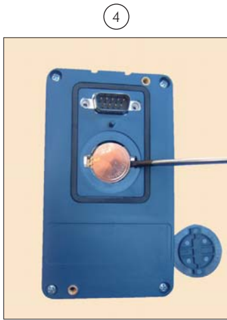
Remove the battery with the help of a screwdriver positioned at the right side
