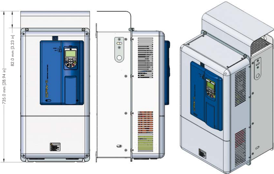
(a) Frame E with the Nema1 kit KN1E-01 - CFW11 0142 T 2 O N1, CFW11 0105 T 4 O N1 and CFW11 0142 T 4 O N1 models
