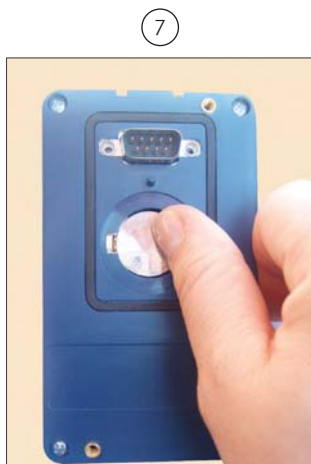
7 Press the battery for its insertion
