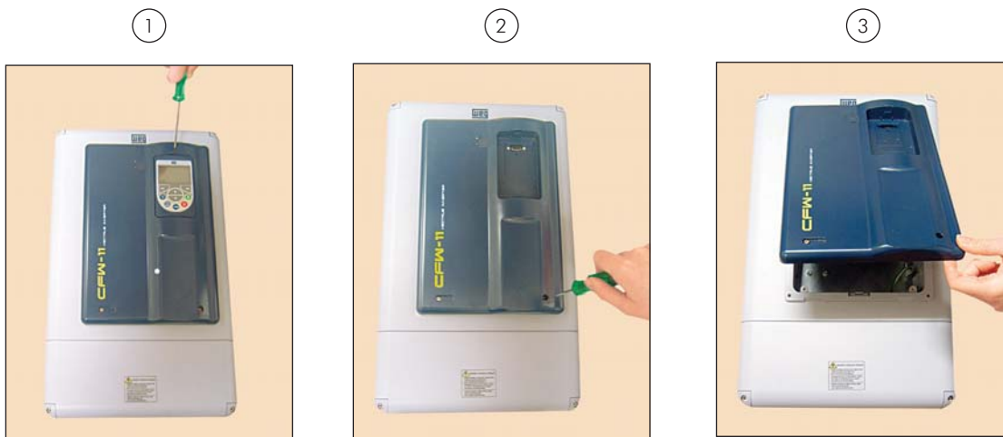
Figure 3.6 - HMI and control rack cover removal
