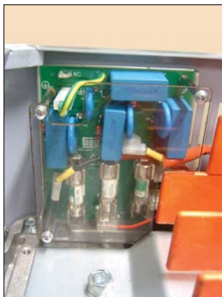
(b) Procedure for disconnecting the RFI filter and the MOV connected to the ground – necessary for using the inverter in IT or corner-grounded delta networks
