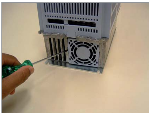
Releasing the latches of the fan cover
