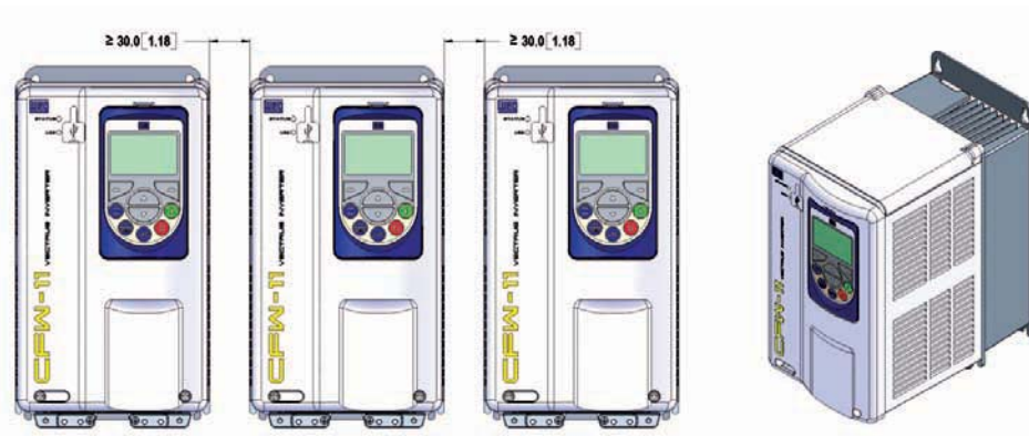
(a) Minimum side clearance requirements
