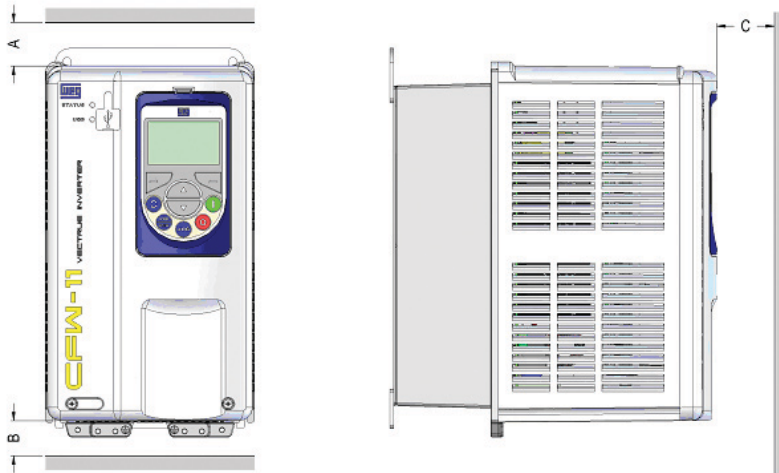
Figure 3.2 - Minimum top, bottom, and front clearance requirements for air circulation
