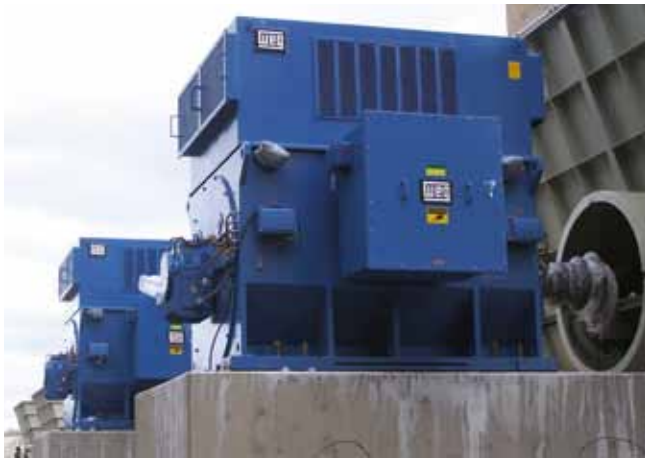
Supply: 9,900 HP, 13,200 V, 8 poles, frame 900 Application: Fan
