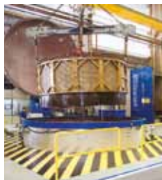
Vacuum impregnation (VPI)
