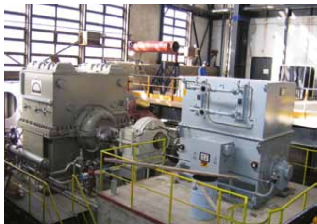
Supply: 12,000 kW, 6,000 V, 4 poles, frame 800 Application: Centrifugal compressor
